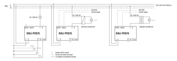
Circuit diagram DALI-PCD/S in DALI- or momentary switch operation
