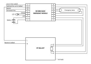
Single lamp high frequency electronic ballast
