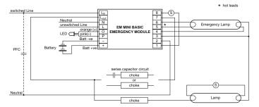
Twin parallel switch start circuit with separate lamp holder and starter holder
