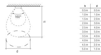
Diameter of the detection cone as a function of height at maximum detection area without taking objects in the room into consideration. Stationary objects (walls, tables, floor-standing luminaires, etc.) located in the direct view of the sensor change the characteristics of the detection area.
