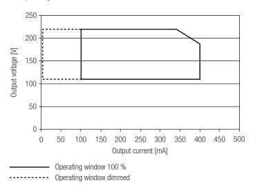
If you run the device outside specification a limitation may be active. This is a technical aspect from the amplitude modulation dimming.
