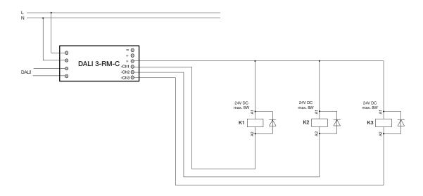
The contactors must be equipped with an appropriate threshold diode. Operation without a threshold diode is not permitted. The controller is designed for a maximum load of 25 W. This load can be split among the three channels. The loads may be distributed asymmetrically.
