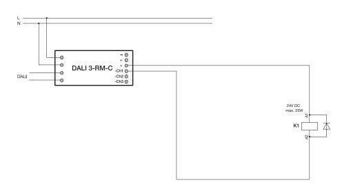
Outputs Ch1 and Ch3 may not be short-circuited. The entire output may flow via one output.
