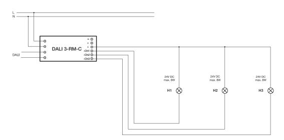
Signal lamps can be connected directly. The controller is designed for a maximum load of 25 W. This load can be split among the three channels. The loads may be distributed asymmetrically.
