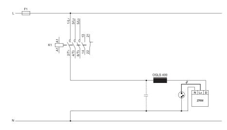
Please check the inrush currents of the switched loads. Electronic control gear may have very high inrush currents. Check with the contactor manufacturer.
