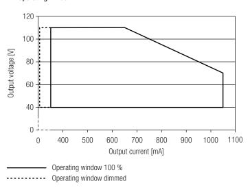
Make sure that the LED Driver is operated within the given window under all operating conditions, also in dimming operation. Otherwise certain limitations may occur. This is due to the nature of amplitude modulation dimming. The stated minimum output voltage shall not be undercut as this may cause the device to shut-down. In this respect, special attention needs to be paid to DC operation.
