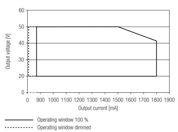
Make sure that the LED Driver is operated within the given window under all operating conditions, also in dimming operation. Otherwise certain limitations may occur. This is due to the nature of amplitude modulation dimming. The stated minimum output voltage shall not be undercut as this may cause the device to shut-down. In this respect, special attention needs to be paid to DC operation.
