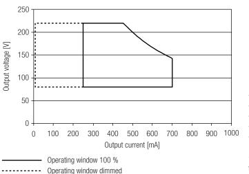
If you run the device outside specification a limitation may be active. This is a technical aspect from the amplitude modulation dimming.
